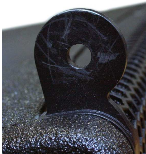
Image 4: Example picture of AiRAY (used) inter-cabinet connection arm
